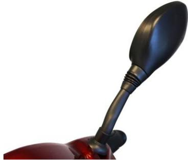
To attach the mirrors simply place each mirror threaded end into the mirror post. Turn mirror clockwise and fasten mirror to scooter.
